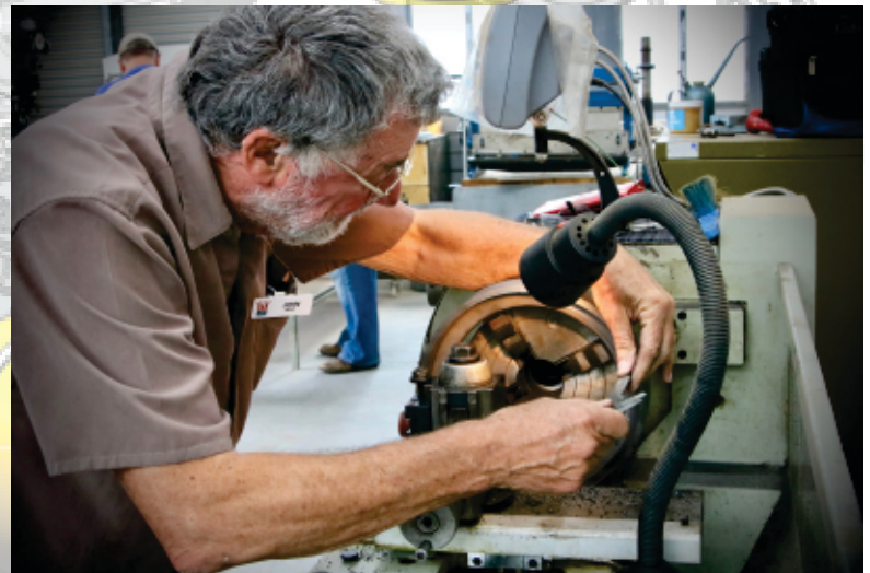
Shed member, John Holt pictured turning a traction engine wheel on the Shed's lathe
